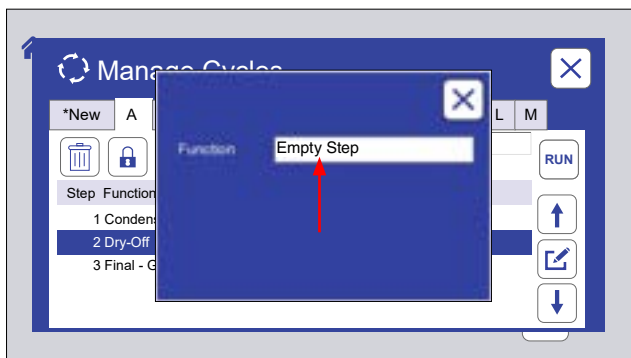
Figure 8.7.4c: Touch the function text box to select a function.
