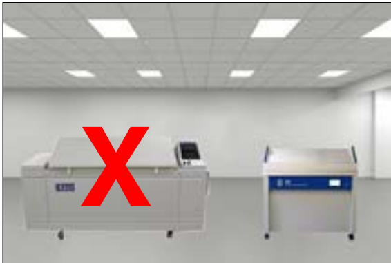
Figure 4.2a: Do not install QCT testers in a room with corrosion chambers.
