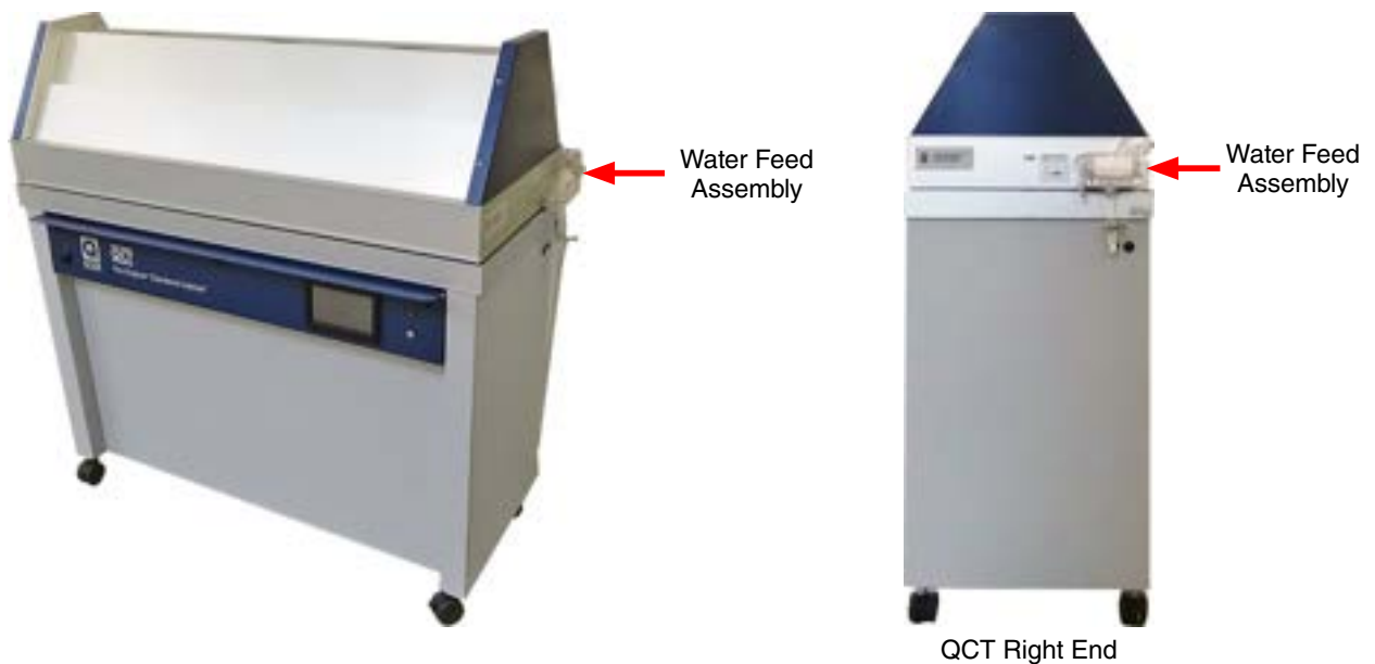
Figure 6.4a: QCT water supply connection location.
