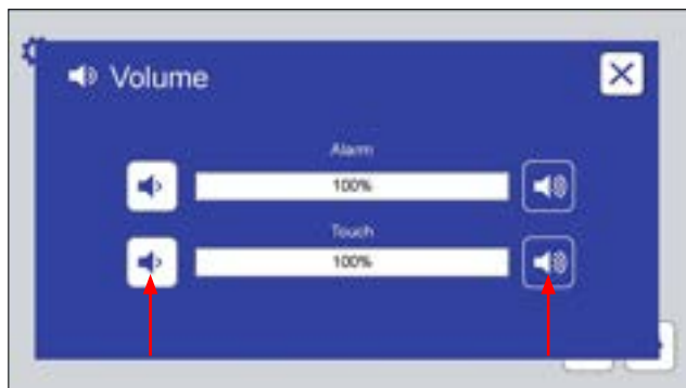
Figure 8.8c: The Volume screen provides controls to set volume (0 to 100) for machine alarms and for the screen touch indicator. Touch a volume icon to adjust.
