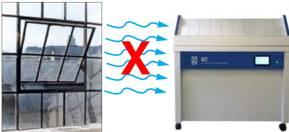
Figure 4.2c: Do not locate the QCT near open windows.
