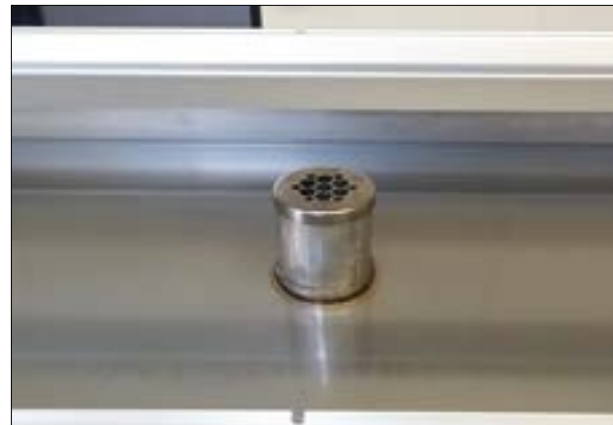
Figure 3.2g: Air heater inside tube at the center of the water pan.
