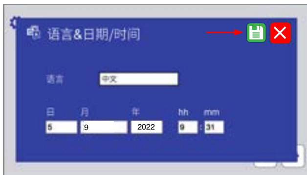
Figure 8.8k: All text on both screens will be in the selected language. Touch the save icon to save the selection.
