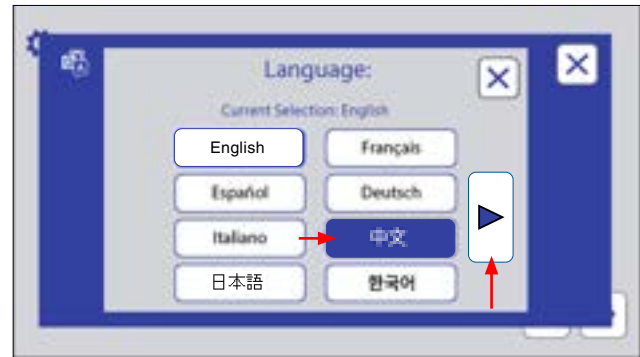
Figure 8.8j: Touch the language text box to select the control display language, or touch the right arrow button to display additional available languages.
