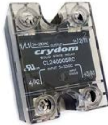
Figure 16.j U-40825-K Relay Kit, SS 5A
