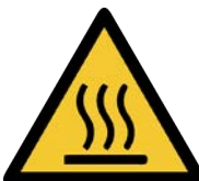
Warning; Hot Surface
