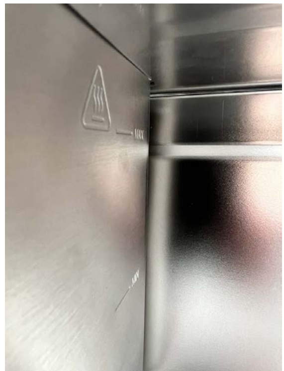
Maximum fill line on the TWB-24NE-4E in relation to the TU-1500
