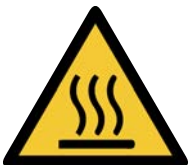
Warning; Hot Surface
